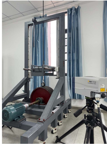
Figure 5. Shimmy test setup for the nose landing gear.
