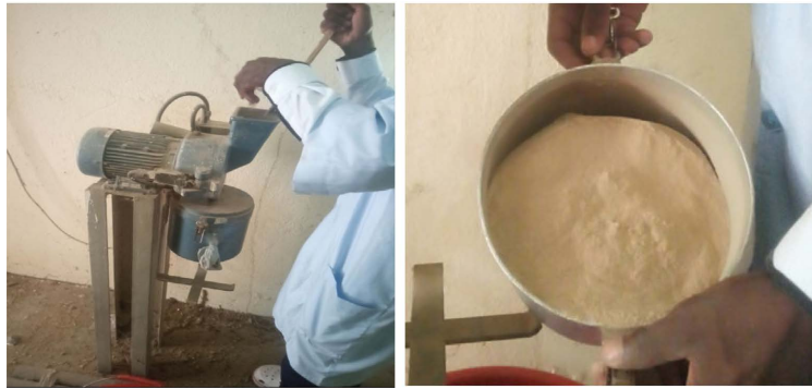
Photo 1. Electric machine for grinding residues into powder.
