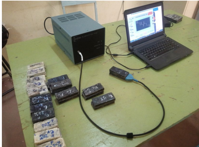
Photo 4. Experimental thermal testing device.
