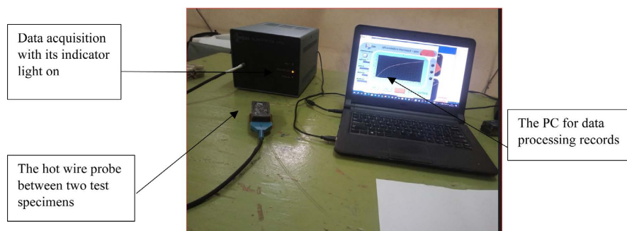
Photo 3. Conducting the thermal conductivity test on the samples.
