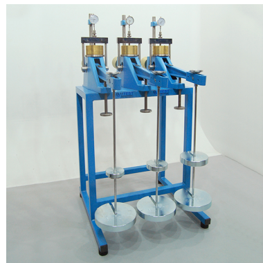
Figure 2. Standard oedometer device.
