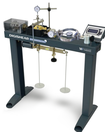
Figure 3. Standard direct shear apparatus.
