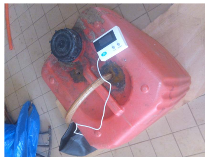
(b) Digester installed in the laboratory with and without adjustment
