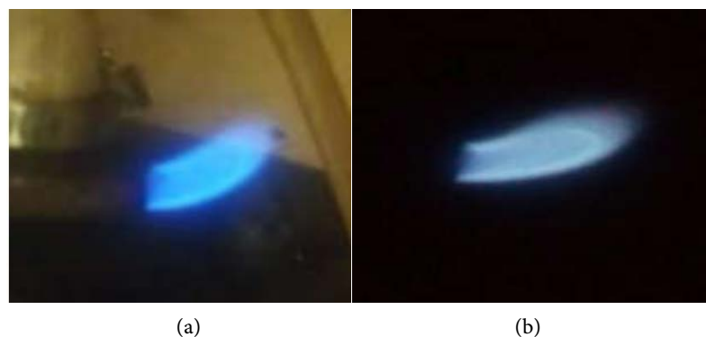
Figure 6. Biogas flammability test.
