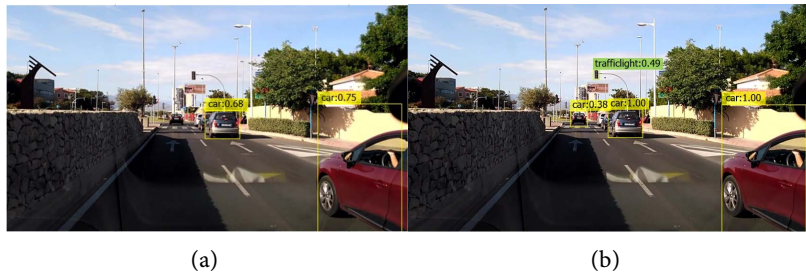
Figure 8. Recognition results obtained by Basic DLOR and the method proposed herein in the fourth frame of scene 4. (a) Basic DLOR; (b) The method proposed herein.
