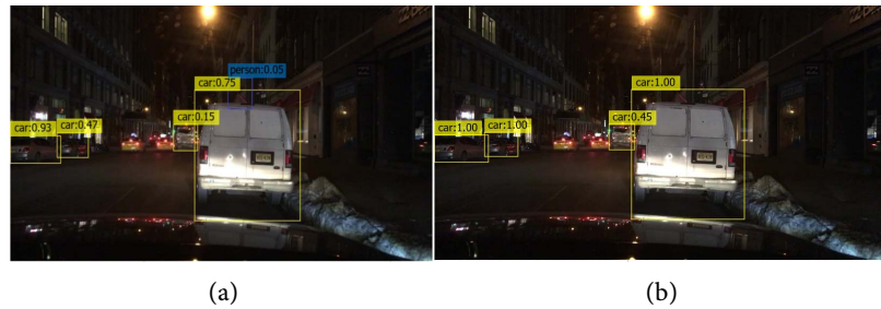
Figure 7. Recognition results obtained by Basic DLOR and the method proposed herein in the seventh frame of scene 2. (a) Basic DLOR; (b) The method proposed herein.
