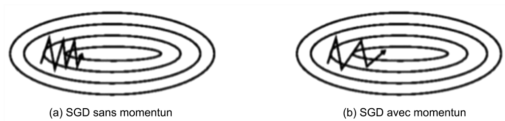
Figure 4. Acceleration and reduction of SGD oscillations by the momentum method.
