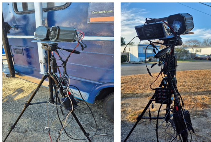
Figure 9. Dual doppler heads, phase pulse shifted 180 degrees, each with a 15-degree azimuth offset.
