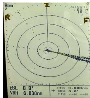
Figure 4. The racon signal displayed on the PPI left shows a radar transponder emitting a characteristic signal when triggered by another ship's radar (Gyyan Staff, 2020) [6].
