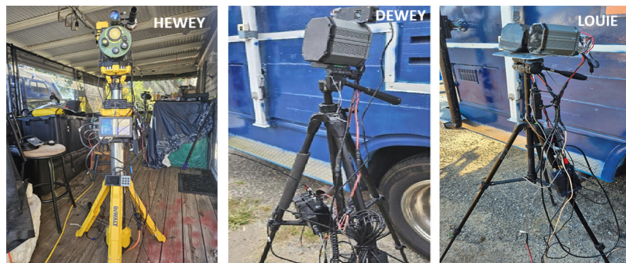
Figure 7. Phase II POD sensors with radar range heads. the PODs from left to right are named, Hewey, Dewey, and Louie.
