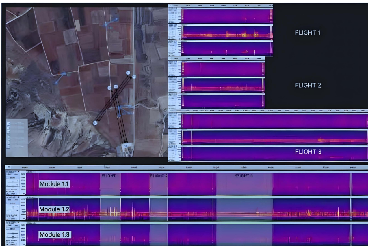
Figure 6. The trajectories of drone flights (upper left figure), their corresponding spectrograms (upper right figure), and a spectrogram of the entire measurement session (lower figure).
