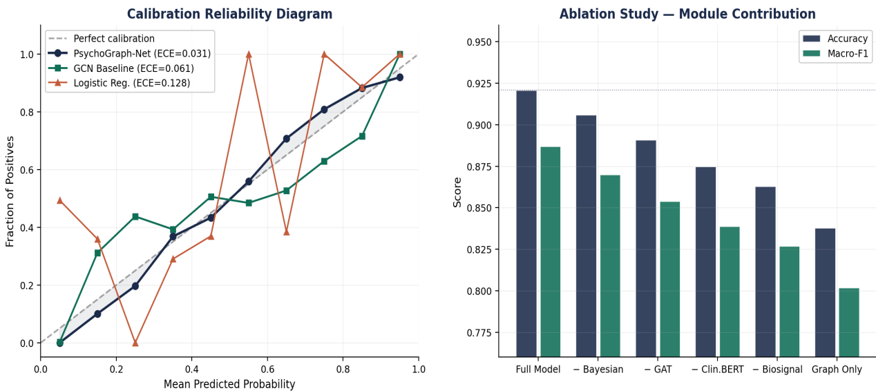
Figure 8. Calibration Reliability Diagram and Module Ablation. Left: PsychoGraph-Net (navy) lies closest to the perfect calibration diagonal (dashed), confirming ECE = 0.031 . Right: Ablation study quantifying the independent contribution of each module. Removing the GAT contributes the largest accuracy drop ( -3.0 pp); removing the Bayesian layer the largest calibration degradation. All modules contribute independently, and their combination yields super-additive benefit.
