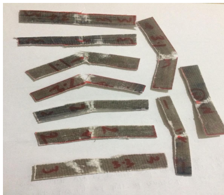
Figure 16. Charpy test specimens.
