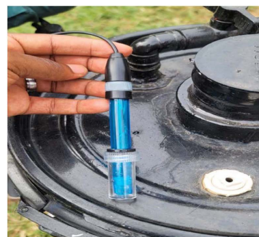
pH sensor to be inserted into the biogas digester
