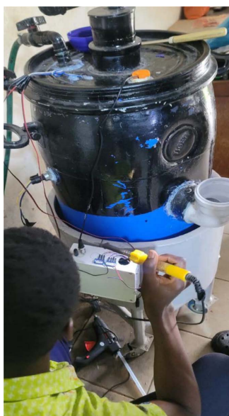
Figure 3. Biogas digester fabrication in progress.
