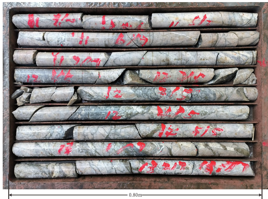
Figure 4. Representative drillhole core photographs from deep ore bodies (illustrating continuous and homogeneous mineralization with gold-bearing pyrite occurring in granular, vein, and disseminated forms within silicified granite).
