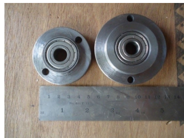
Figure 14. Bearings of gear assembly.
