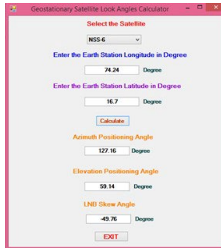
Figure 21. C# GUI for look angle calculation.
