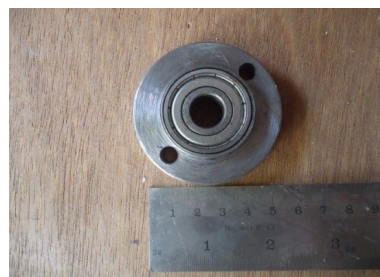
Figure 10. Actual designed bearing.
