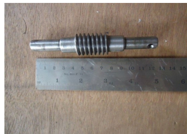
Figure 8. Actual designed worm.
