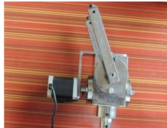
Figure 17. EL assembly for antenna positioner.
