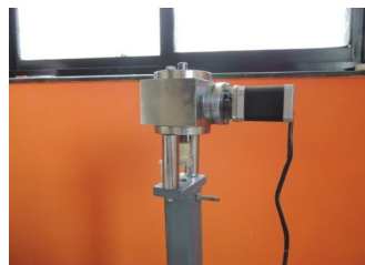
Figure 18. Az assembly for antenna positioner.
