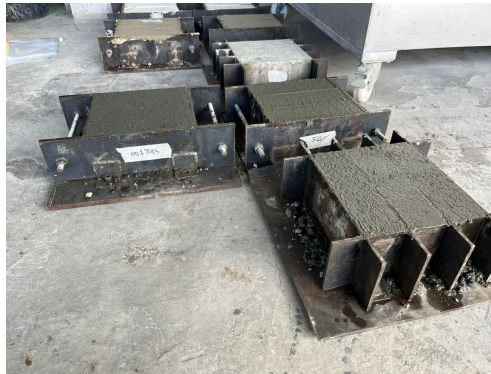
Figure 2. Casting of paver block.
