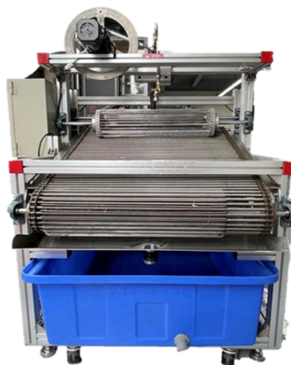
Figure 1. The developed hydraulic fiber extraction and degumming machine.
