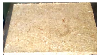
Figure 5. Particleboard of Andropogon gayanus .
