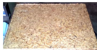
Figure 6. Particleboard of Sorghumbicolor.
