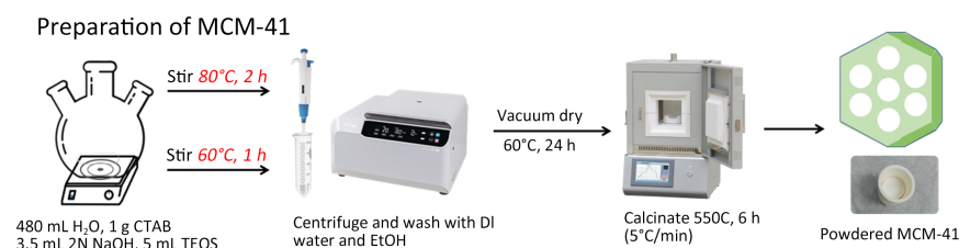
Figure 2. Schematic illustration of preparation of MCM-41.
