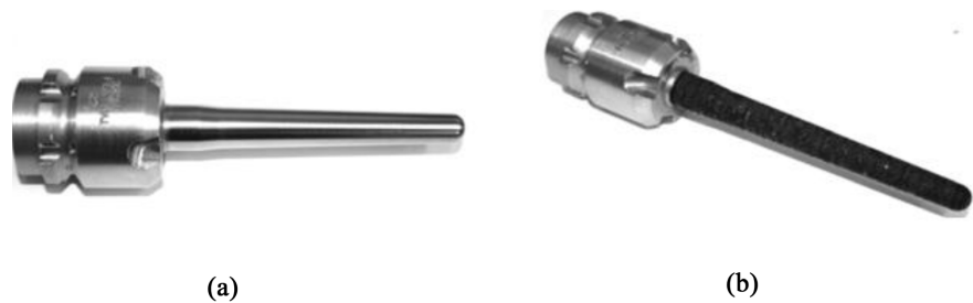
Figure 15. General view of the punch surface of the plunger of the glass casting molds: (a) Initially; (b) After machining [37].
