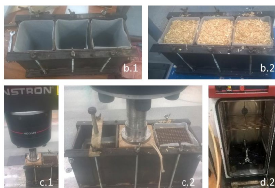
Figure 1. Steps in manufacturing composites by molding.
