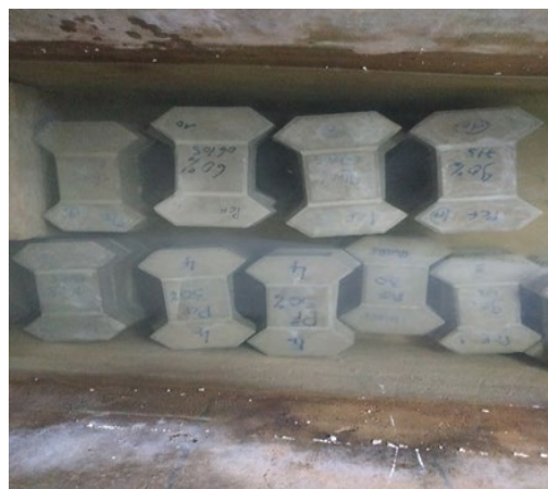
Figure 3. Paving stones placed in a tank of water.
