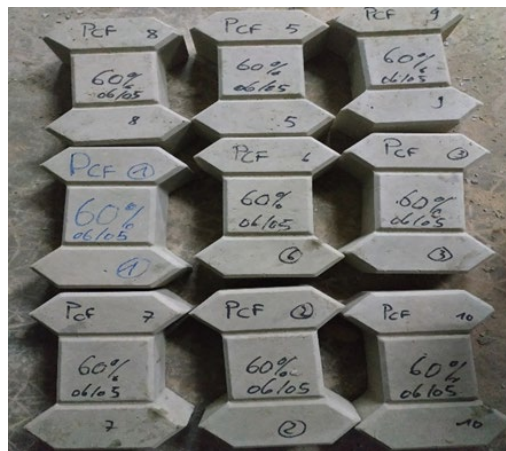
Figure 2. Paving stones unmolded after 24 hours.
