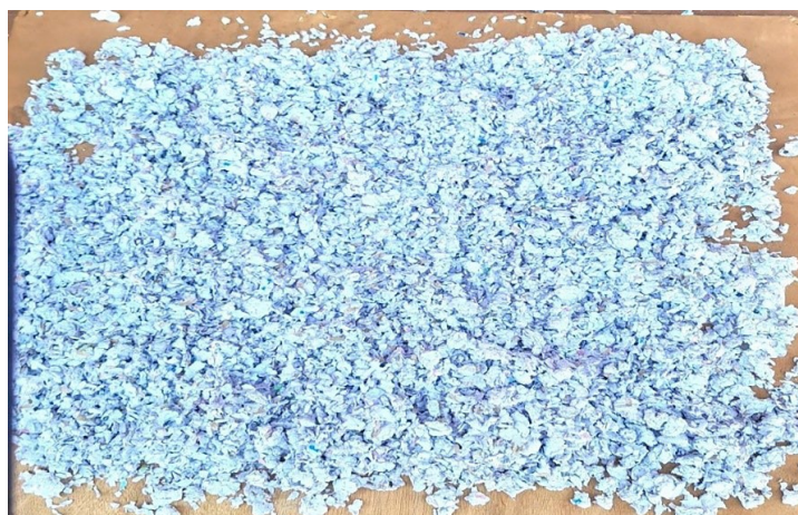
Figure 4. Showing the cellulose fibers of recycled paper after grinding and soaking in water for 24 hours.
