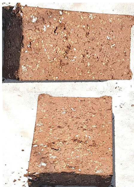
Figure 3. Examples of mud brick samples stabilized with shredded paper.
