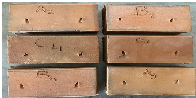
Figure 1. Specimens of platelets made from waste coal fly ash and gray clay.
