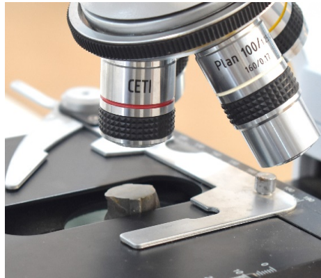
Figure 6. The positioning of the iron sample piece in the microscope.
