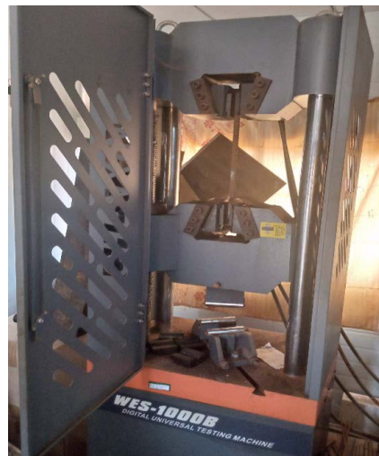
Figure 4. Tensile and flexure apparatus showing the device.
