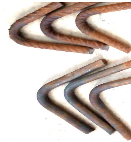
Figure 5. Showing the iron bars after V-shaped bending.
