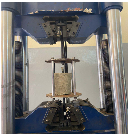
Figure 4. Experimental setup for the pull-out test.
