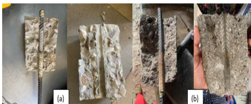
Figure 10. Facies after rupture for cementitious concrete (a) and PET (b).
