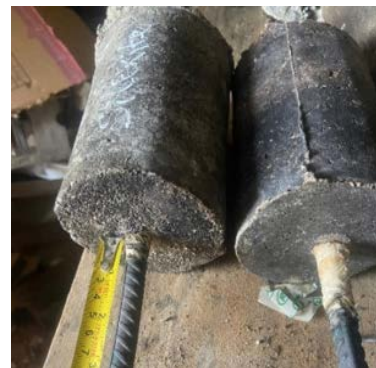
(b) rupture by sliding
