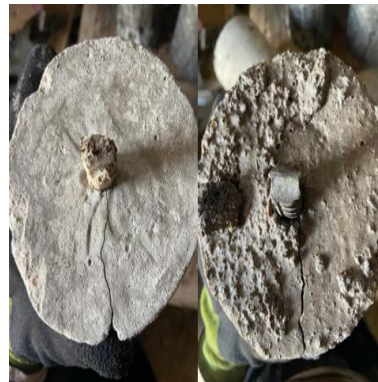
(a) rupture by bursting
