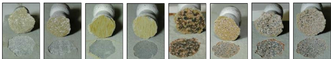
Figure 5. Evaluation of coating adhesion using the pull-off method.
