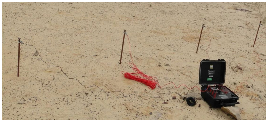
Figure 10. Wenner method for soil resistivity determination in a Brazilian wind park.
