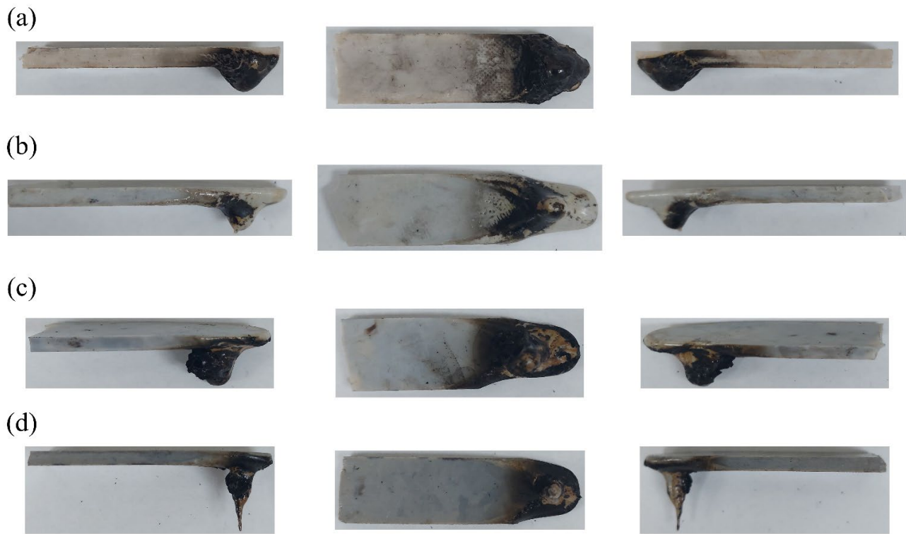
Figure 15. FS appearance after flammability test: (a) FS1, (b) FS2, (c) FS3 and (d) FS4; from left to right: right side view; bottom side view and left side view.
