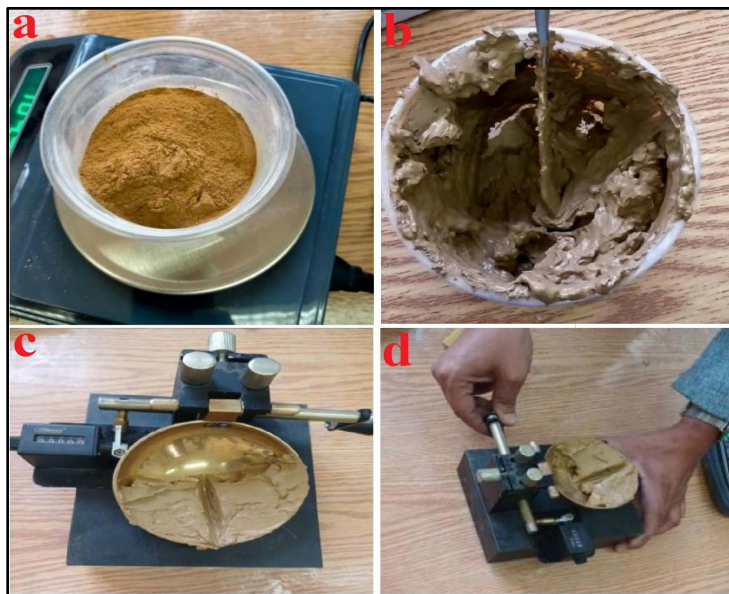
Figure 4. Steps for performing the Atterberg limit test. (a) Weight of the dry soil. (b) The sample is mixed with a suitable amount of water. (c) A portion of the mixture is placed in the front part of the casagrande device. (d) Turn on the device, which operates at a rate of two blows per second.
