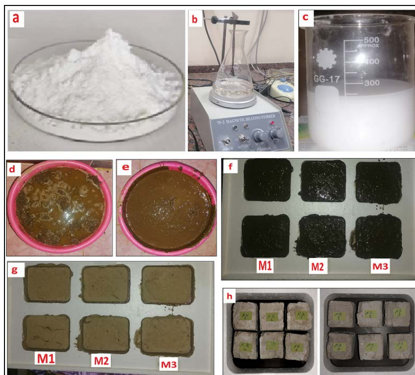
Figure 3. (a) \text{Ca}(\text{OH})_2 Nanoparticles. (b) (c) \text{SiO}_2 nanoparticles. (d) Clay washing stage (this stage is done several times). (e) Clay fermentation stage (leaving for 28 days). (f) The stage of clay forming into blocks of regular dimensions. (g) The mud brick blocks after drying. (h) The mud brick blocks after cut into cubes with dimensions of ( 4 \times 4 \times 4 \text{ cm}^3 ).
