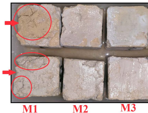
Figure 5. The new mud brick specimens during partial immersion in salt solution, M1 show swelling and cracks in mud brick surface, and M2 and M3 show accumulation of salt on bricks surface.
