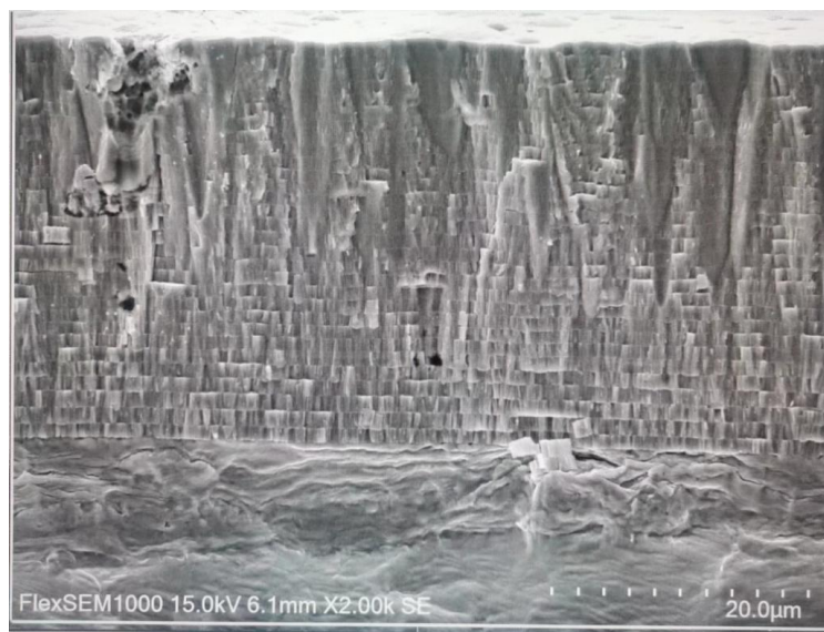
Figure 4. Fracture morphology of chromium nickel composite coating.
