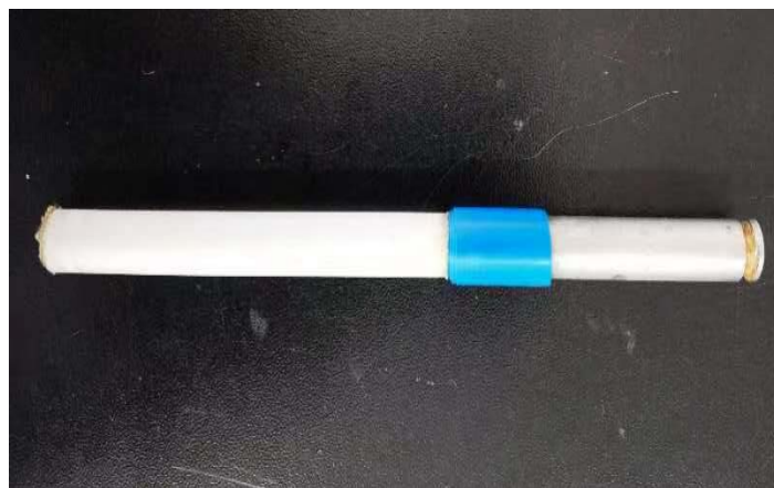
Figure 8. Chromium-nickel composite coating on 30CrMnSi steel with upper, middle, and lower thickness of eighty microns, seventy microns and one hundred microns, respectively.
