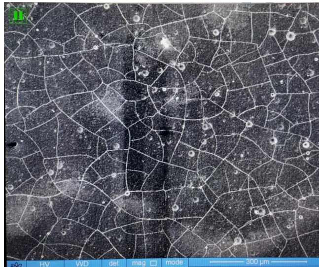
Figure 7. Microcrack metallography of Cr-Ni composite coating.
