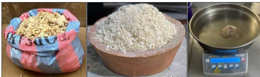
Figure 3. Process of obtaining sugarcane bagasse ash.
