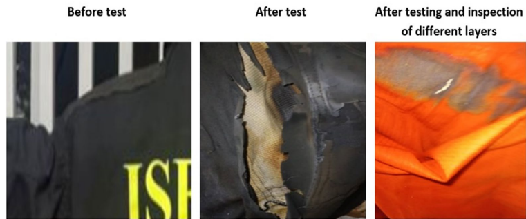
Figure 14. Photograph of the intervention suit, shoulder part before and after FPP test.
