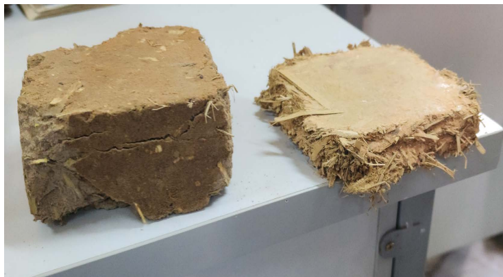
Figure 19. Appearance of a sample of raw earth + crushed palm leaf fibers before and after compression.
