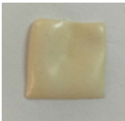
Figure 2. Sample (10 mm × 10 mm) used for swelling test.
