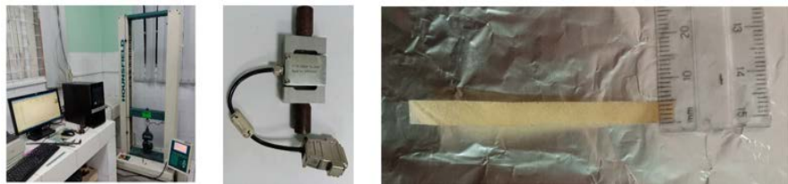
Figure 3. Equipment and sample (60 mm × 5 mm) used for mechanical test.
