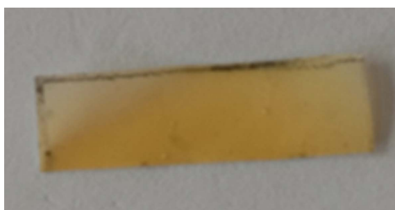
Figure 1. Sample (5 mm × 2 cm) used for porosity test.
