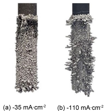
Figure 4. Photographs of Zr deposits on graphite substrate in LiF-NaF-ZrF 4 (1.96 mol·kg -1 ) at 750 °C at two current densities: -35 (a) and -110 (b) mA·cm -2 .
