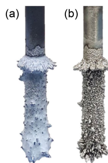
Figure 2. Typical Zr deposit on graphite cathode (a) before and (b) after ultrasonic cleaning.
