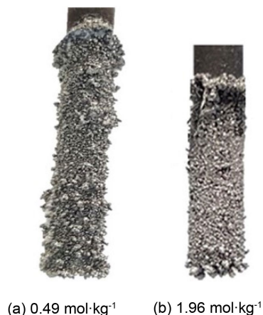
Figure 3. Photographs of Zr deposits on graphite substrate at -0.035 \text{ A}\cdot\text{cm}^{-2} for 5 h in LiF-NaF-ZrF 4 at 750 °C for 0.49 (a) and 1.96 (b) mol·kg -1 of Zr(IV).
