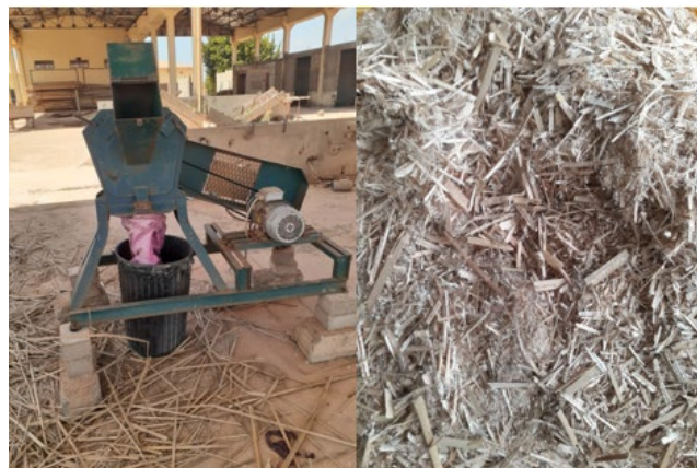
Figure 2. Crusher and ground Typha.
