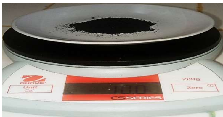
Figure 7. Pretreated lead paste on a mass balance 10 g.
