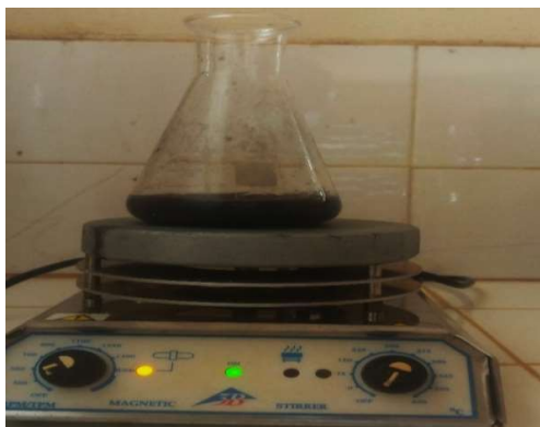
Figure 8. Photograph of the first stage of leaching of lead paste on a magnetic shaker (black solution).
