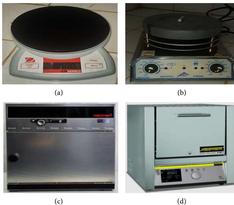
Figure 4. Laboratory equipment. (a) Precision balance (Maximum load 200 g, sensitivity 0.1 mg), (b) magnetic stirrer (speed continuously adjustable from 0 to 2000 rpm., Plate diameter: 120 mm.), (c) Air oven (Voltage: 230 V, 50 - 60 Hz, Power: 600 W, Content: 14 L, Temperature range: 220°C), (d) Electric oven (Volume: 15 liters, Max temperature: 1200°C).
