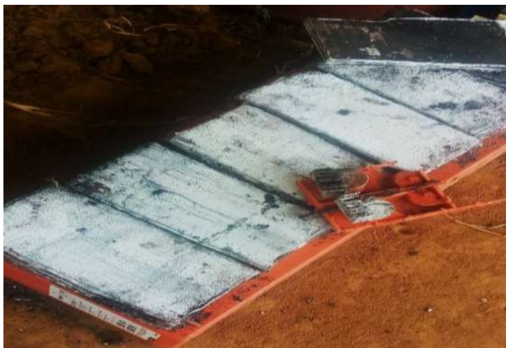
Figure 5. Photograph of the dismantled battery.
