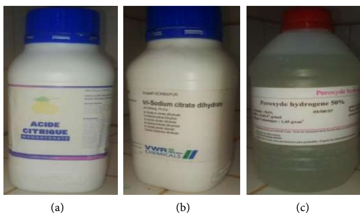
Figure 3. Chemical reagents. (a) Bottle containing crystals of hydrated citric acid ( C_6H_8O_7 \cdot H_2O ) with a purity of 98%, (b) Vial containing crystals of sodium citrate hydrate ( Na_3C_6H_5O_7 \cdot 2H_2O ) with a purity of 98%, (c) Bottle containing a 50% purity hydrogen peroxide solution.
