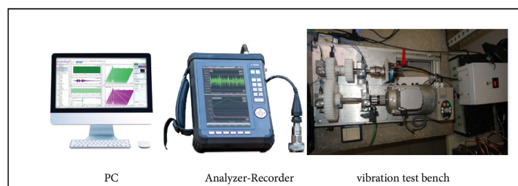
Figure 1. Data acquisition equipment and National Instruments CoCo-80X vibration analyzer.
