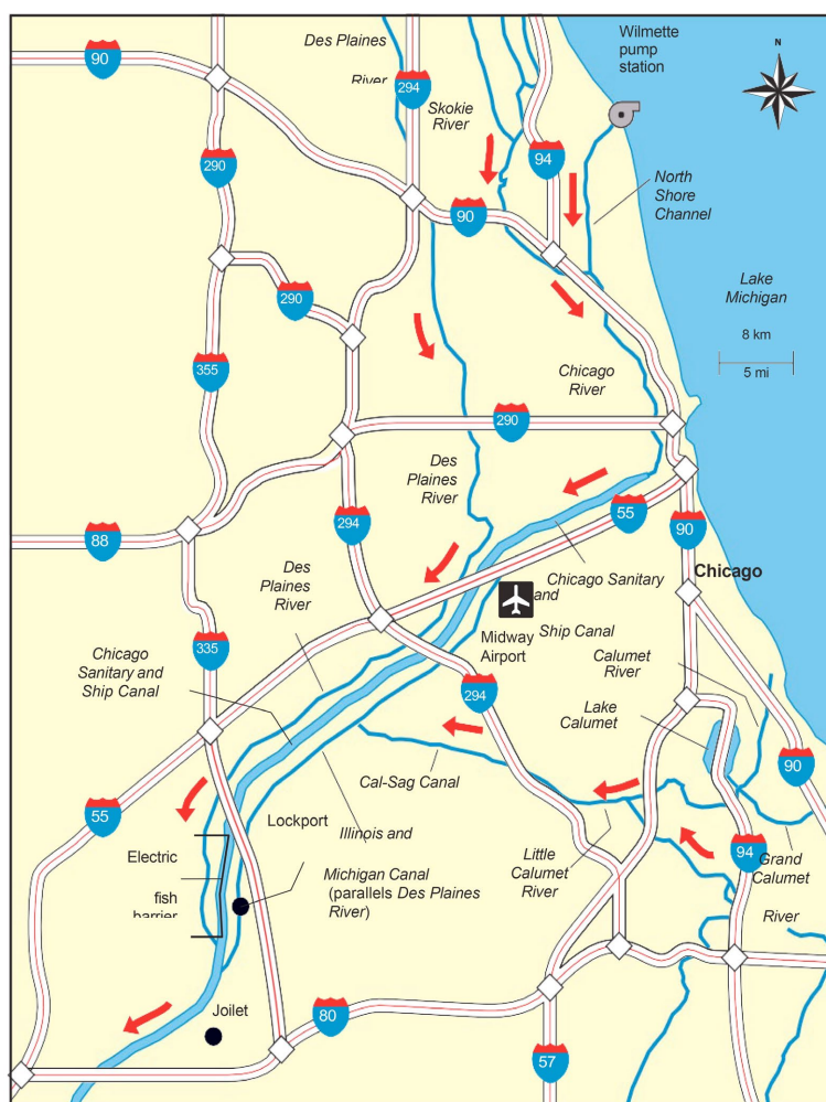
Figure 4. This 2015 map shows the direction of the water in the Chicago canals after the Chicago and Calumet rivers were reversed to carry wastewater away from Lake Michigan into the Chicago Sanitary and Ship Canal and south into the Illinois Waterway and the Mississippi River [2].
