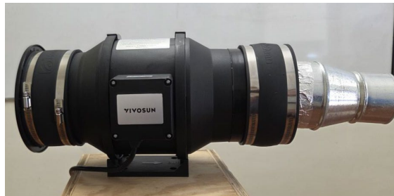
Figure 1. A custom-built controlled wind apparatus was used to simulate wind conditions. The system includes an eight-vane, 6-inch diameter fan powered by a 120-volt electric motor (2450 RPM), generating airflow up to 390 CFM. Wind speed was adjusted via a variable resistor and measured with a HoldPeak® HP-866B anemometer.
