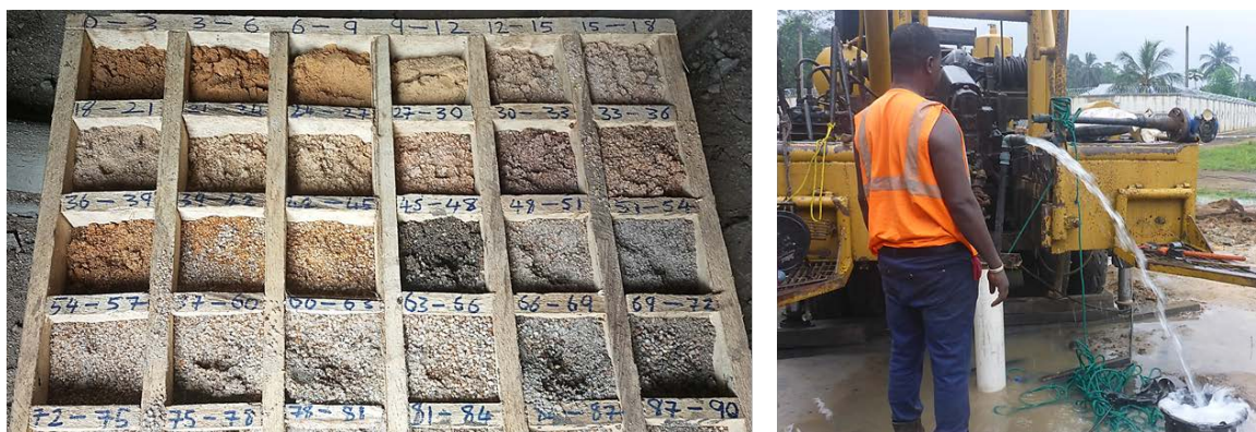
Figure 8. Fine to coarse grained Coastal Plain Sand (left) and borehole yield estimation during pumping test.
