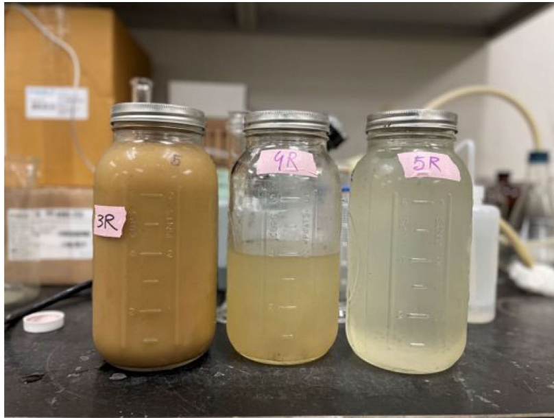
Figure S4. Collected runoff samples from bare soil (control cases), class IV, and EQS biosolids (left to right).
