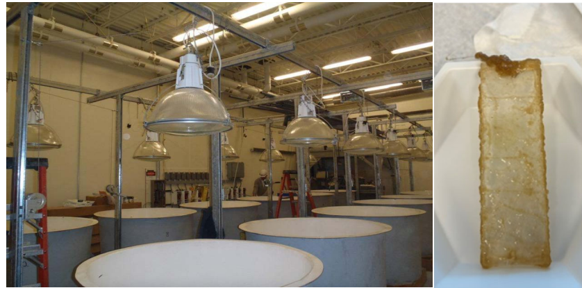
Figure 1. Left: AWRI mesocosm facility showing tanks and metal halide lamps suspended above them; right: periphyton-colonized strip after two weeks of deployment in the control treatment.
