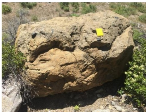
Figure 6. Palagonitized hydrovolcanic tuff boulder. The dimensions of this boulder are d_1 = 3.40 m, d_2 = 2.75 m [12]. Field notebook for scale ( \sim 14 cm \times 20 cm). Cliffs formed of this lithology are present within 0.3 km of this boulder exposed in the quarry.
