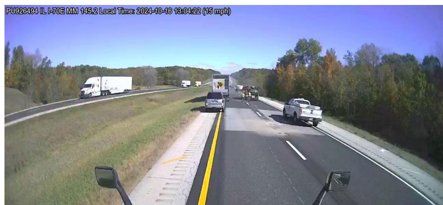
Figure 7. Dash camera image along I-70 in Illinois showing shoulder running of several vehicles due to lane incursions from work crew.
