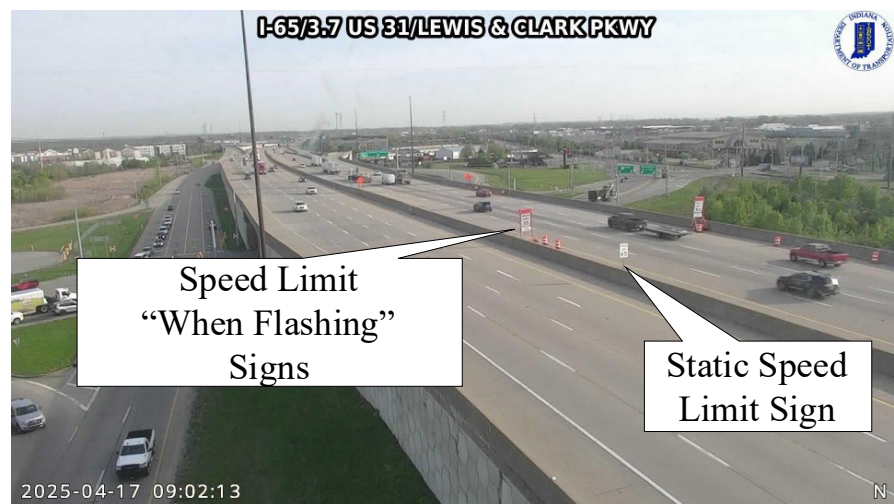
Figure 1. ITS camera image on I-65 in Indiana showing a static speed limit sign and a work zone speed limit trailer in close proximity.
