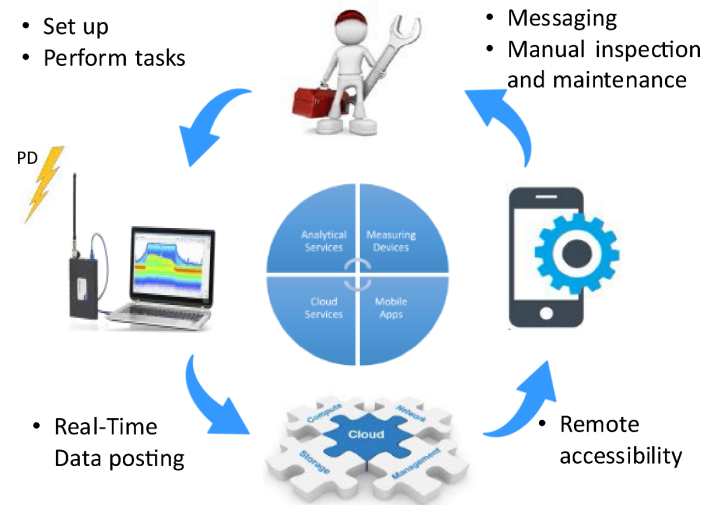
Figure 3. IoT-cloud-based remote accessible real-time PD monitoring system diagram.
