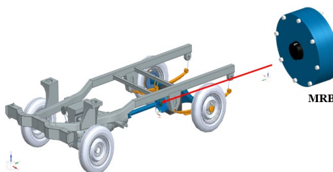
Figure 1. Layout of the magnetic brake on a small truck.
