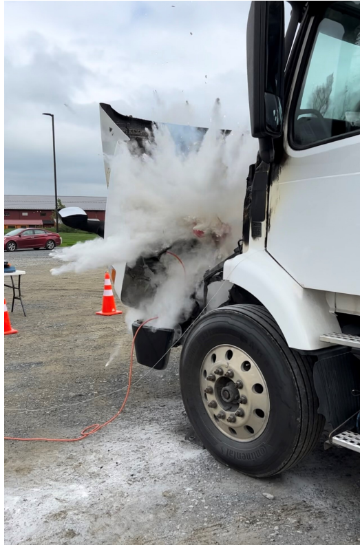
Figure 2. Photo showing the blast of monoammonium phosphate (MAP) powder.
