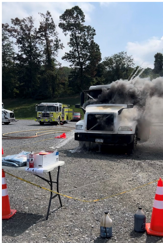
Figure 3. Photo showing the engine on fire with the truck's hood closed at the moment of ignition.
