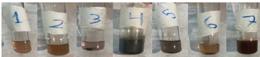
Figure 3. The samples after Silver Mirror Test (Tollens' Test for Silver Nitrate).
