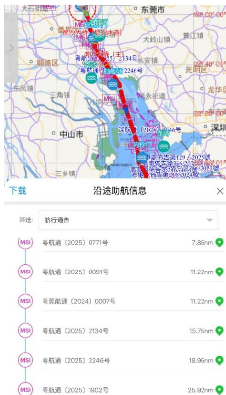
Figure 7. Visual display of S-124 navigation warnings in the APP, along with push notifications of navigation warnings along the planned flight route.
