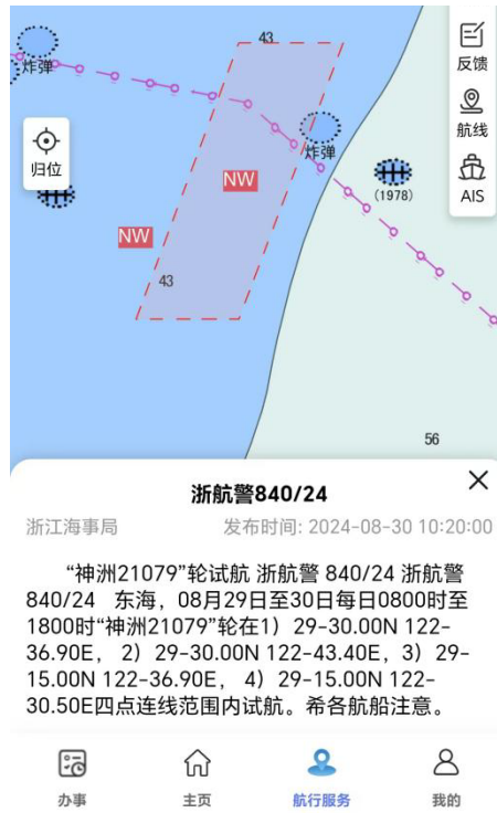
Figure 6. Visual display of S-124 navigation warnings in the APP, along with push notifications of navigation warnings along the planned flight route.
