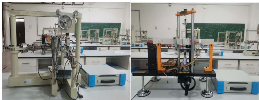
Figure 3. Multi-functional composite test bench of material mechanics.
