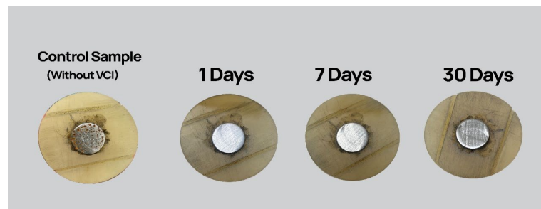
Figure 4. German standard TL-8135-0043: Corrosion Evaluation of Samples Without VCI and Protected with VCI Formulation (1, 7, and 30 days).
